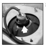
2. Turn the bulb/socket retainer (arrow) counterclockwise to unlock the bulb/socket. You may prefer to unplug the electrical connector before removing the bulb/socket. If so, complete Step 4 before doing this step.
